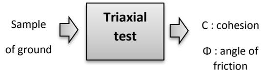
Figure 9: Objective of the triaxial test
