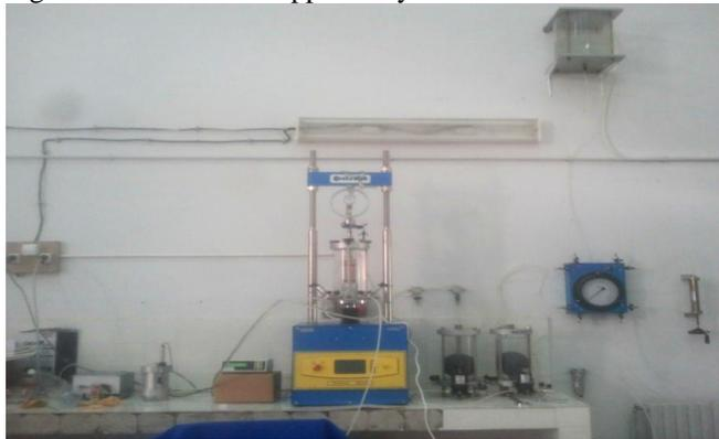
Fig. 15. An overview of triaxial appartus system
