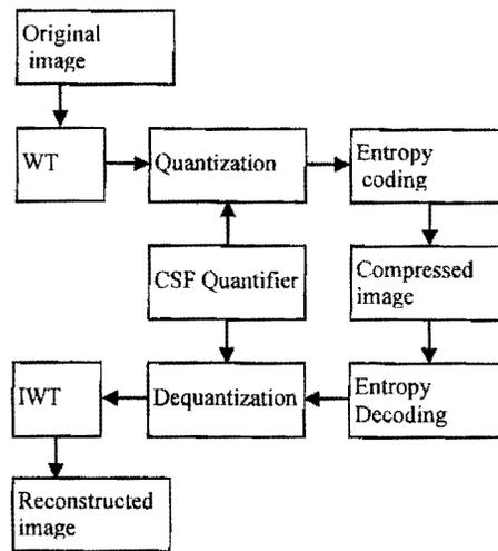
*Figure 3: The incorporation of the CSF Quantifier*
