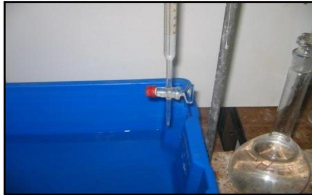
Fig 2. Correction of the sulfate solution by adding small quantities of 0.1N  $H_2SO_4$ , up to a pH equal to 6-8.
