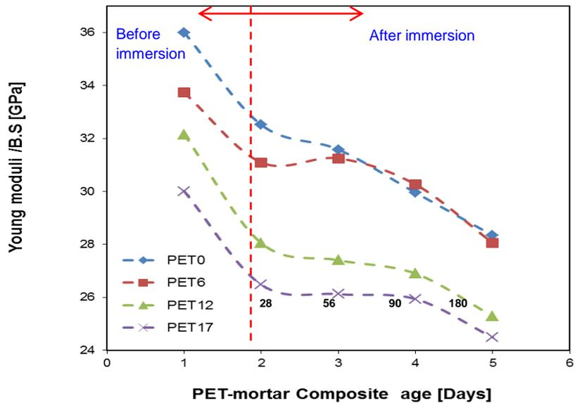
Fig 4. Evolution of Young modulus with volumetric PET rate and composite mortar ages via BS-8110 code before and after MgSO<sub>4</sub> attacks
