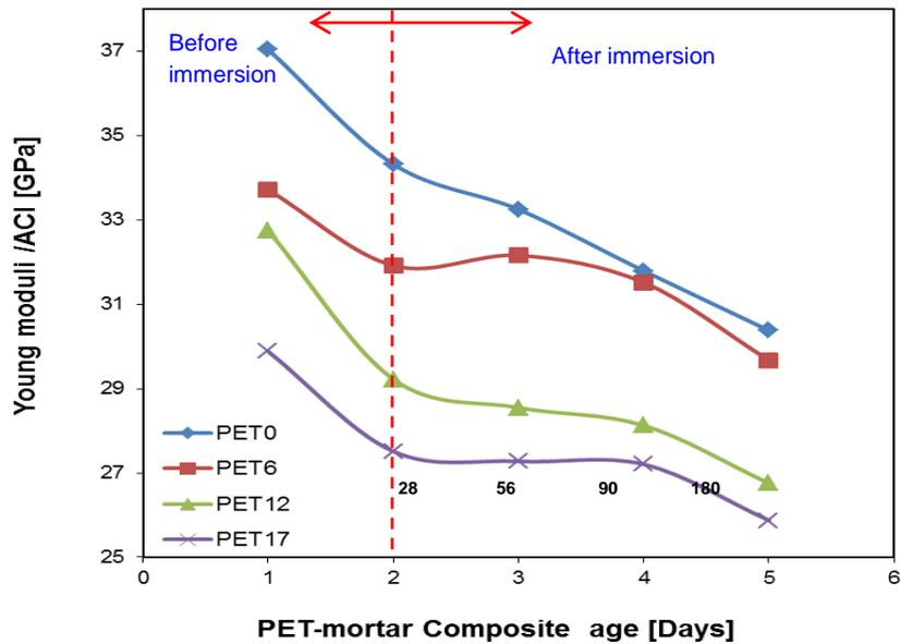
Fig 3. Evolution of Young modulus with volumetric PET rate and composite mortar ages via ACI-318 code before and after MgSO<sub>4</sub> attacks
