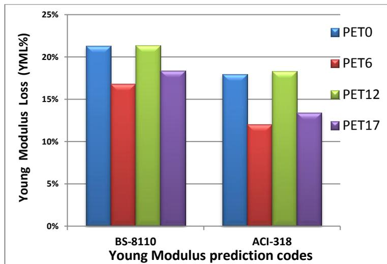
Fig 5. Young modulus loss (YML%) with volumetric PET rate and prediction codes (BS-8110 & ACI-318) before and after  $MgSO_4$  immersion
