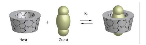
Fig. 3. Cyclodextrins structure and inclusion complex formation [20].
