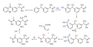
Fig. 8. Proposed UV photolysis pathway of KD.
