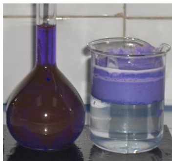
Fig. 7 – Dye mixture solution containing MB, RhB, MG and BR29 before and after extraction by ELM under most favorable experimental conditions (the concentration of each dye in the mixture is 10 mg/L).
