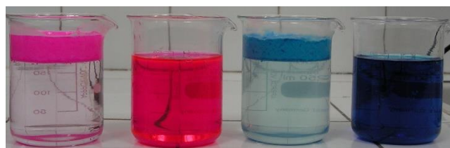
Fig. 5 – MB and RhB solutions (10 mg/L) before and after extraction by ELM under most favorable experimental conditions.
