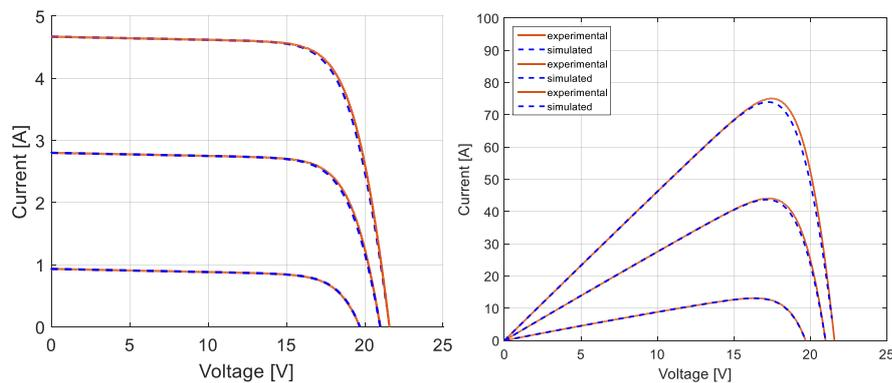
Figure 6. and P-V characteristics obtained by our model and experimental data at three different irradiances (200W/m<sup>2</sup>, 600W/m<sup>2</sup> and 1000W/m<sup>2</sup>).
