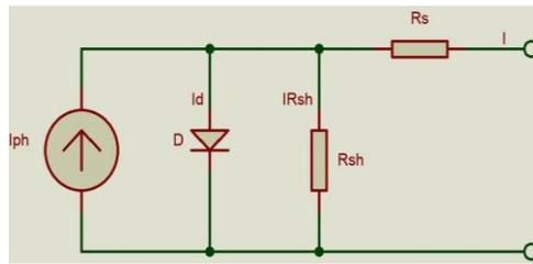
Figure 1. Equivalent circuit for PV cell
