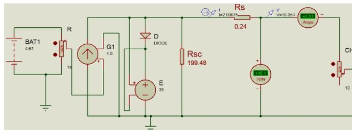
Figure 4. Equivalent circuit of a photovoltaic panel for measuring the I-V characteristic.
