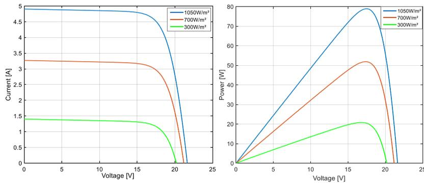
Figure 5. The I-V and P-V simulation results of the isfetone 75W module; according to the solar irradiation for a fixed temperature of 25°C
