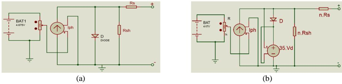
Figure 3. PV cell and panel model implemented under ISIS-Proteus software, (a) PV cell model, (b) PV panel model
