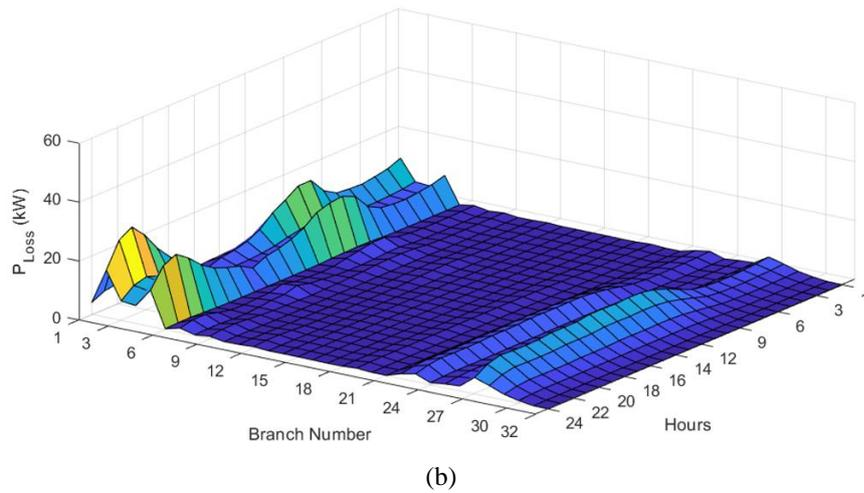
Figure 6. The daily variation of active power losses for distribution system.
