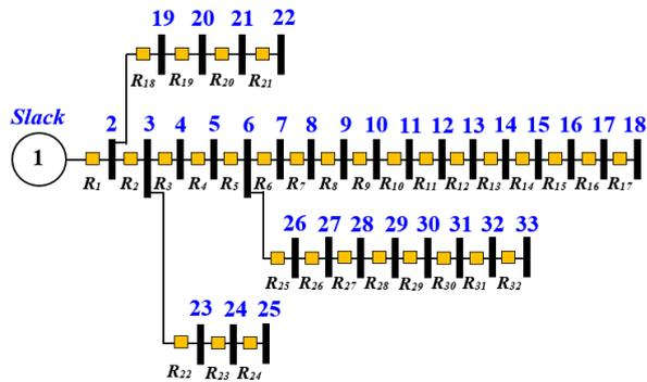
Figure 4. Single diagram of IEEE 33-bus distribution system.
