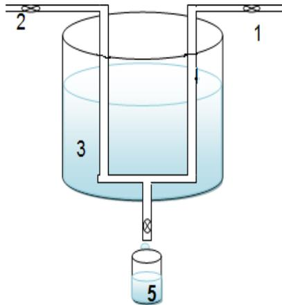
(1) Arrival of hydrated biogas; (2) Take out dehydrated biogas; (3) Ice water; (4) U shape copper tube; (5) Water recovery.
