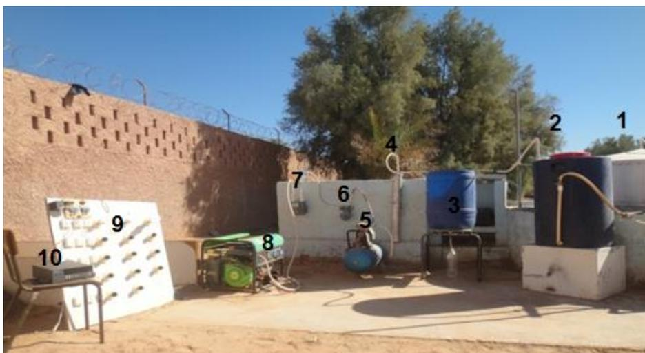
(1) Digester; (2) CO<sub>2</sub> filter; (3) Water trap; (4) H<sub>2</sub>S filter; (5) Air compressor; (6) Regulator; (7) Gas meter; (8) Gas generator; (9) Load table; (10) Data acquisition.
