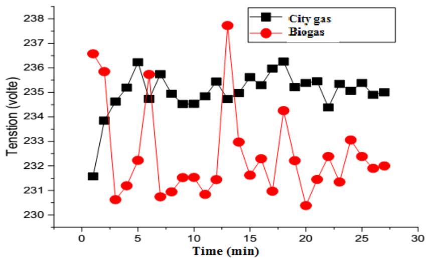
Figure 8. Recording of the voltage of the electric current with the town gas and our biogas.
