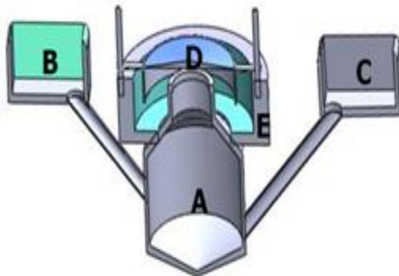
A: Digestion tank; B: Feeder tray; C: Digesta evacuation tank; D: Gasometric bell; E: Gasometer basin
