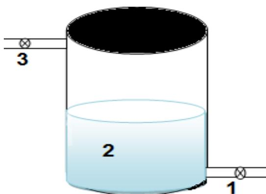
(1) Arrival of biogas; (2) lime water; (3) Exit biogas
