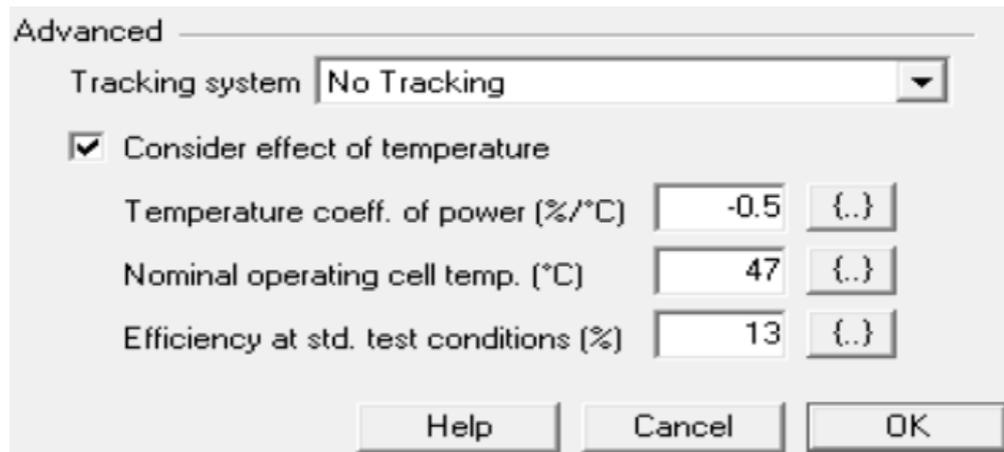
Figure 5. Effect of temperature by HOMER.
