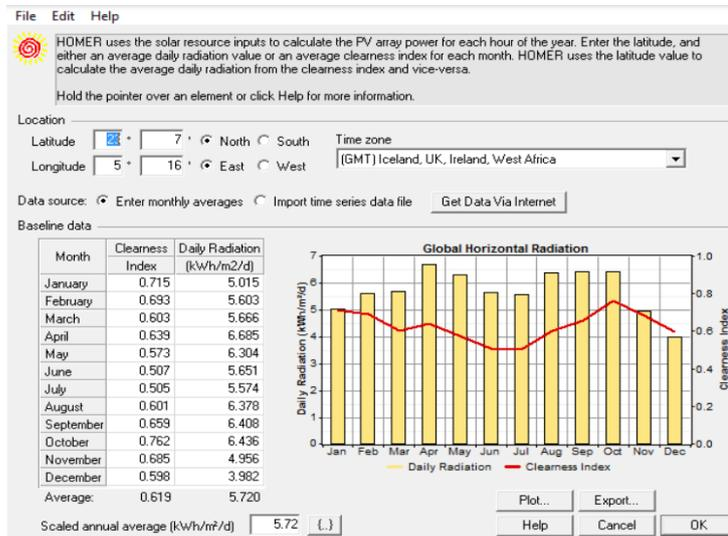
Figure 9. The irradiance data of the installation site.
