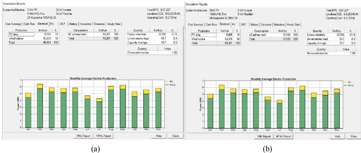
Figure 13. Optimal techno-economical results for extrapolated wind speed data following, (a) Power law 1/7, (b) Logarithmic law.
