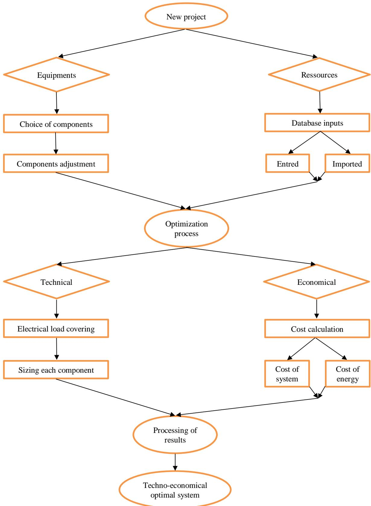
Figure 7. Flowchart of the optimization process on HOMER.
