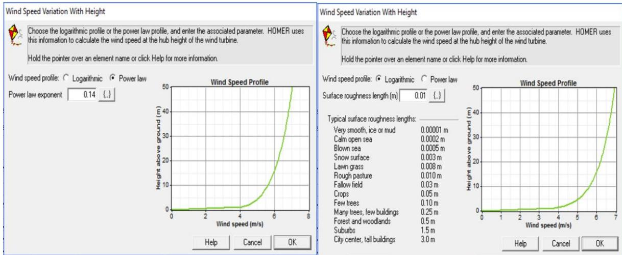
Figure 12. Wind speed variation with height following, (a) Power law 1/7, (b) Logarithmic law.
