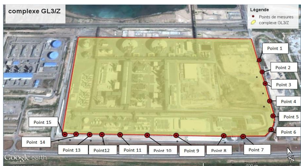
Figure 4. Limited Battery noise measurement positions for the LNG3/Z complex.
