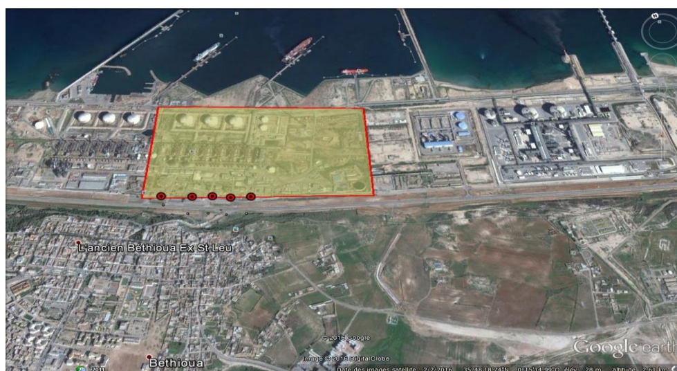
Figure 6. Limited Battery noise measurement positions for the LNG2/Z complex
