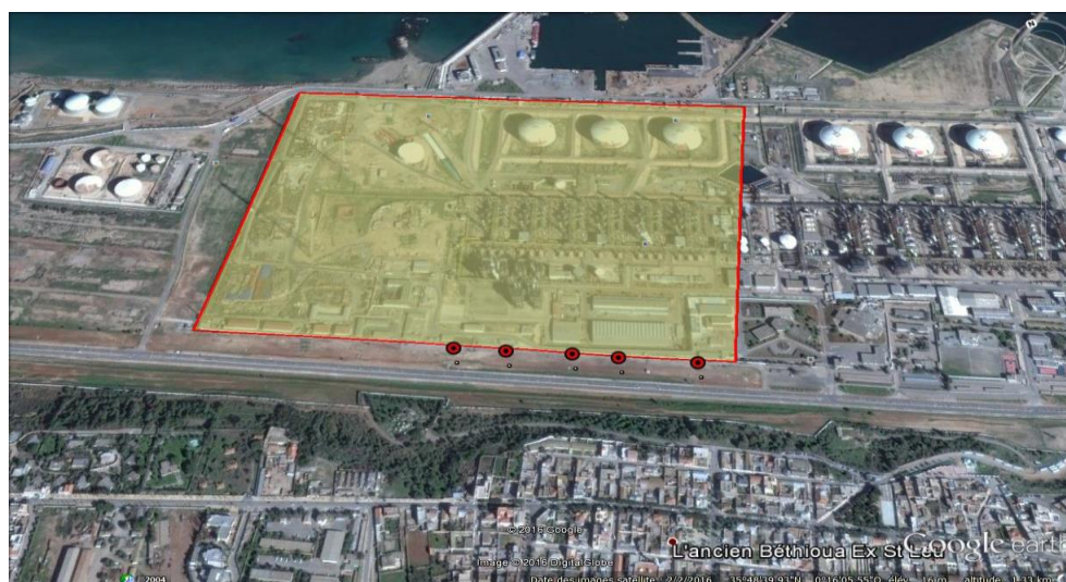
Figure 5. Limited Battery noise measurement positions for the LNG3/Z complex.
