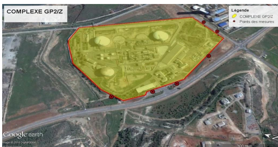
Figure 3. Limited Battery noise measurement positions for the GP2/Z complex.
