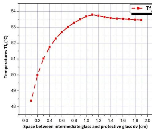
**Figure 7 :** Variation of the fluid temperature as a function of the air space  $esp_{v2v1}$ .
