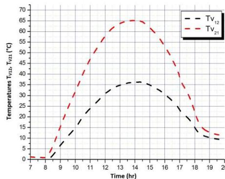
**Figure4:** Temperature variation of protecting glass  $T_{v12}$  and the temperature of the intermediate glass  $T_{v21}$
