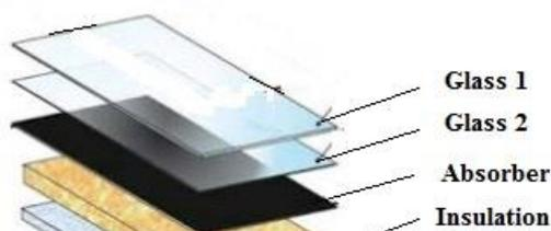
**Figure2:** Double glazing collector components.
