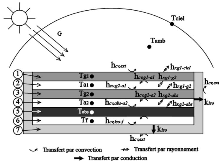
**Figure 1** Representation of the double-glazing flat plate solar collector [7]
