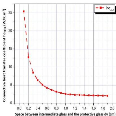
**Figure 6 :** Variation of the  $h_{c-v2v1}$  convection exchange coefficient as a function of the air space  $esp_{v2v1}$ .
