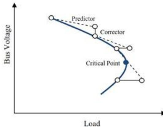
Figure 3. Predictor-corrector scheme of the continuation power flow [15].
