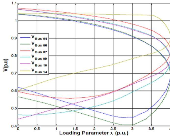
Figure 8. P-V curves of sensitive bus bars.
