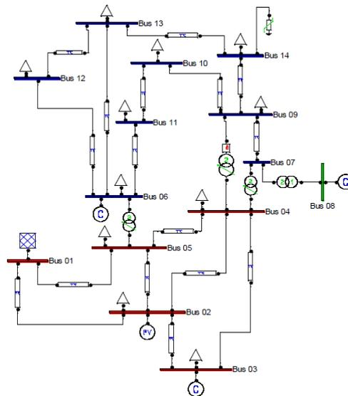
Figure 5. Integration of a SVC at busbar n°14 in a network of 14 busbars.
