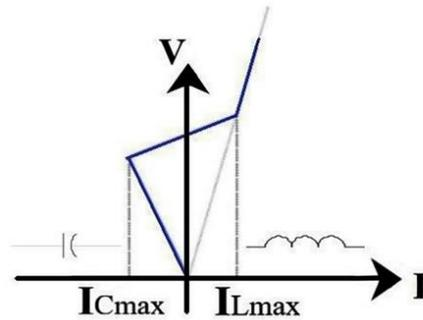
Figure 2. Characteristic of an SVC.
