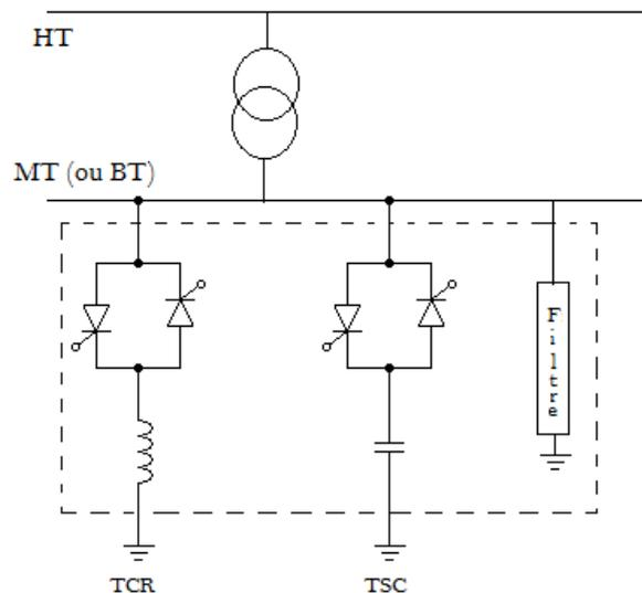
Figure 1. SVC (Static Var Compensator).
