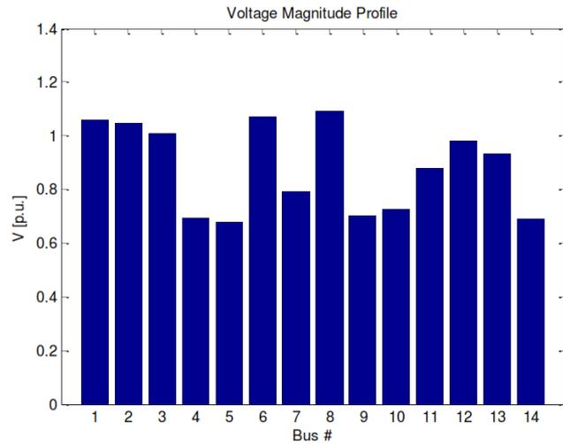
Figure 6. Voltages of 14 bus bars network without SVC.
