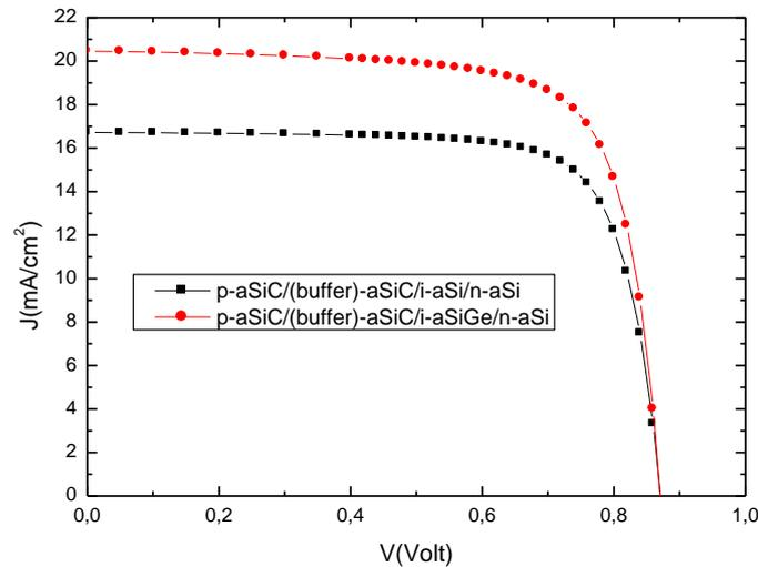
Figure 3: Simulated J–V characteristics of solar cells.
