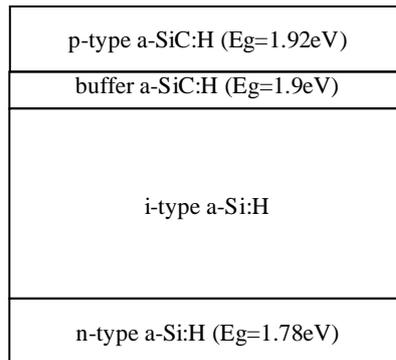
Fig. 1. Structure of p-i-n single-junction solar cell based on a-Si:H alloys: (a) a-SiC:H as window layer (p and buffer layer),
