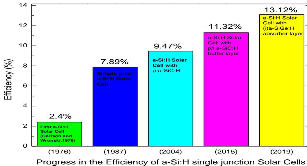
Figure 5: Progress in the efficiency of a-Si:H single junction solar cell since first solar cell 1976,
