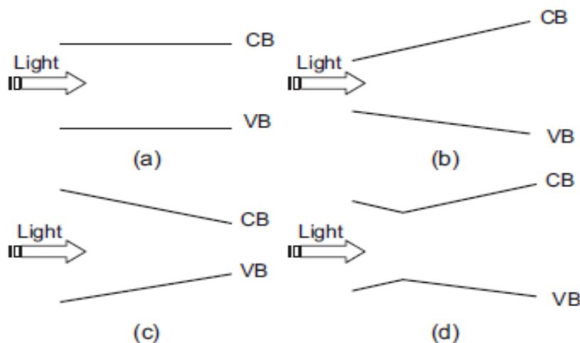
Figure 2: Schematics of bandgap Engineering in a-Si:H solar cells [18]
