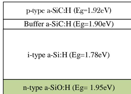
Figure 4. Design of a-Si:H p-i-n solar cell structure with n-type a-SiO:H layer
