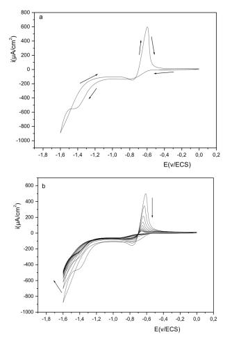
Fig. 1. Electrodeposition of indium on an n-Si (111) electrode (S =  $0.30 \text{ cm}^2$ ) at v = 0.1 V/s and pH = 3, a: one cycle, b: repetitive scanning
