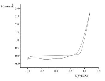
Fig. 2. Cyclic voltammogram of an n-Si (111) electrode in CH<sub>3</sub>CN 10<sup>-1</sup>M LiClO<sub>4</sub> and  $4x10^{-3}$  M Pyrrole, at v = 0.1V/s.
