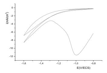
Fig.5. Electrodeposition of indium on n-Si/polypyrrole by scanning at v = 10 mV/s after immersion in a solution of indium chloride  $8x10^{-3}$  M, for 20 minutes.
