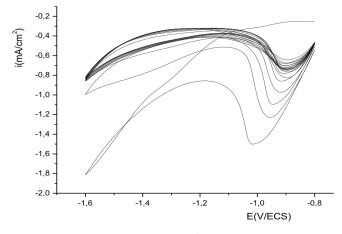
Fig. 4. Direct electrodeposition of indium on polypyrrole/n-Si, with v: 10m V/s and pH =3.
