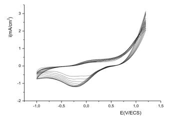
Fig. 3. Repetitive scanning electropolymerization of pyrrole on n-Si (111).
