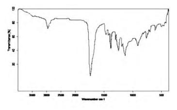
Fig 1. FT-IR spectrum of poly(ethylene succinate).
