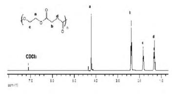
Fig. 2. Nuclear magnetic resonance (1H NMR) spectra of poly(ethylene succinate).
