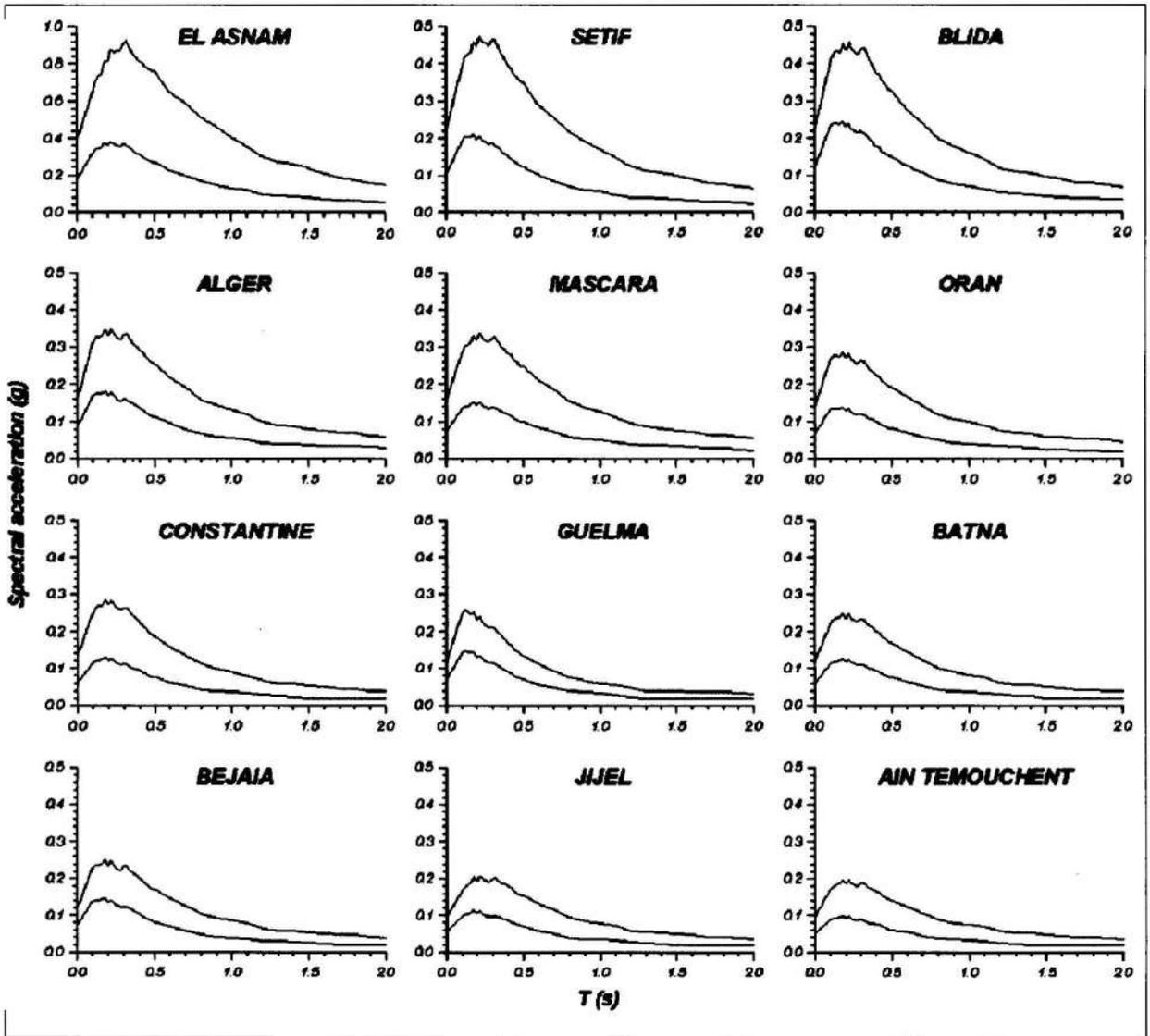
Fig. 9 - UHS (for rock and 5% damping) with 39.3% and 10% probability of exceedance in 50 years for 12 selected cities in northern Algeria. The unit of the y-axis is in g ( $g \approx 10m/s^2$ )
