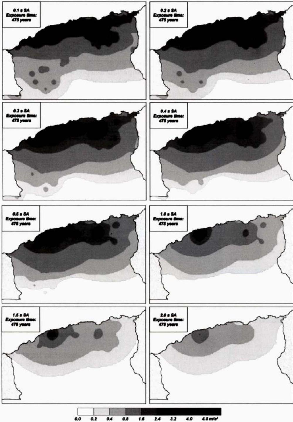
Fig. 8 - Seismic hazard in terms of SA for rock and 5 % damping at different period 0.1 to 2.0s for a return period of 475 years.
