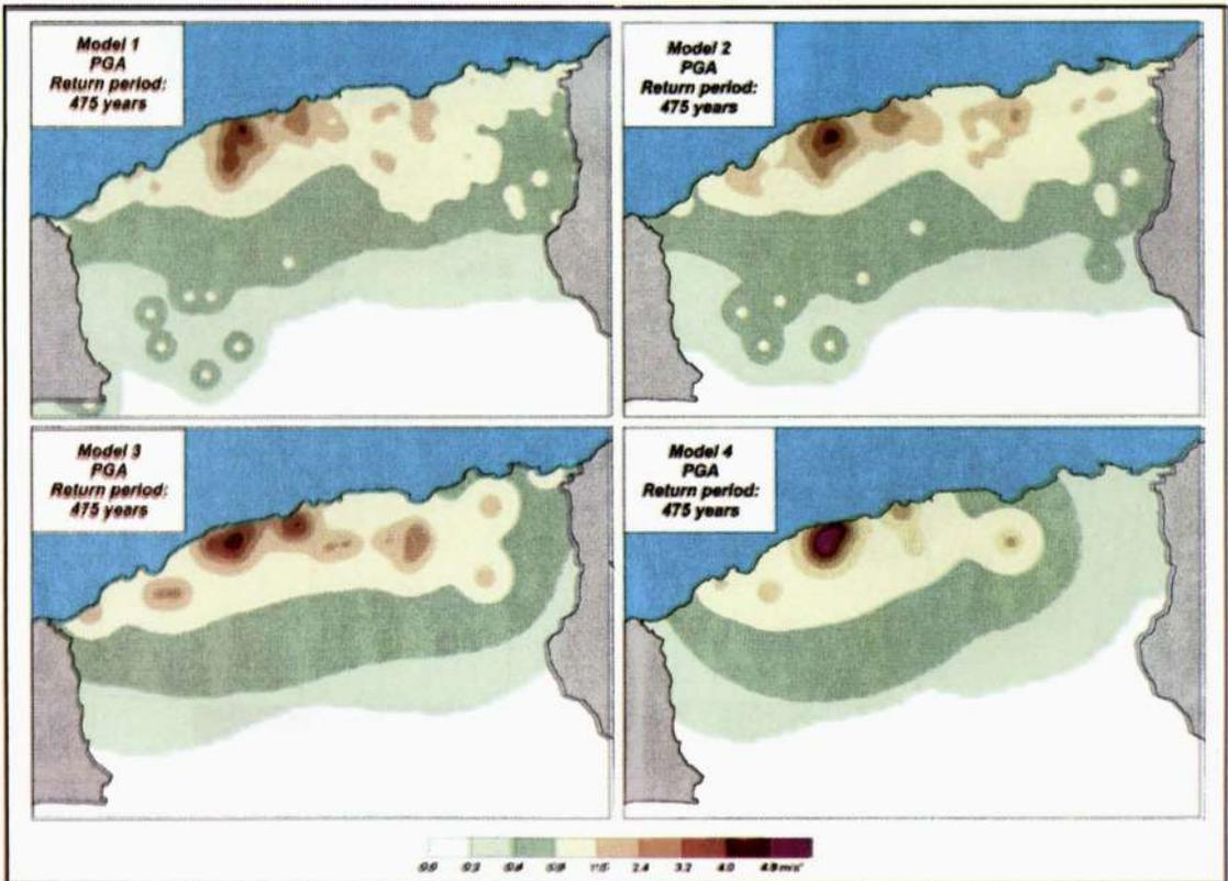
Fig. 5 - Seismic hazard maps in terms of PGA for a return period of 475 years, for the four seismic models.
