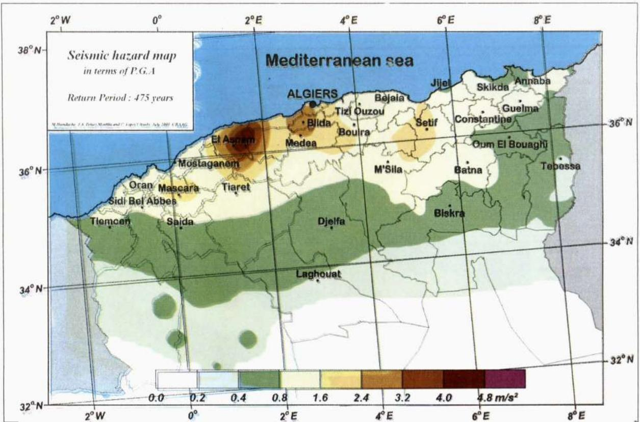
Fig. 6 - Seismic hazard map for northern Algeria in terms of PGA acceleration with 10 % probability of exceedance in 50 years.
