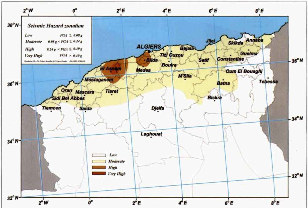
**Fig. 7 - Seismic hazard zoning in northern Algeria.**
