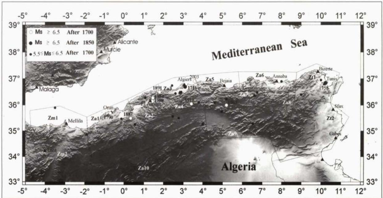
Fig. 3 - Seismicity map showing  $5.5 \leq M_s < 6.5$  (small gilled circles) and  $M_s \geq 6.5$  (large gilled circles) earthquakes since 1850 and  $M_s \geq 6.5$  (large open circles) since 1700.
