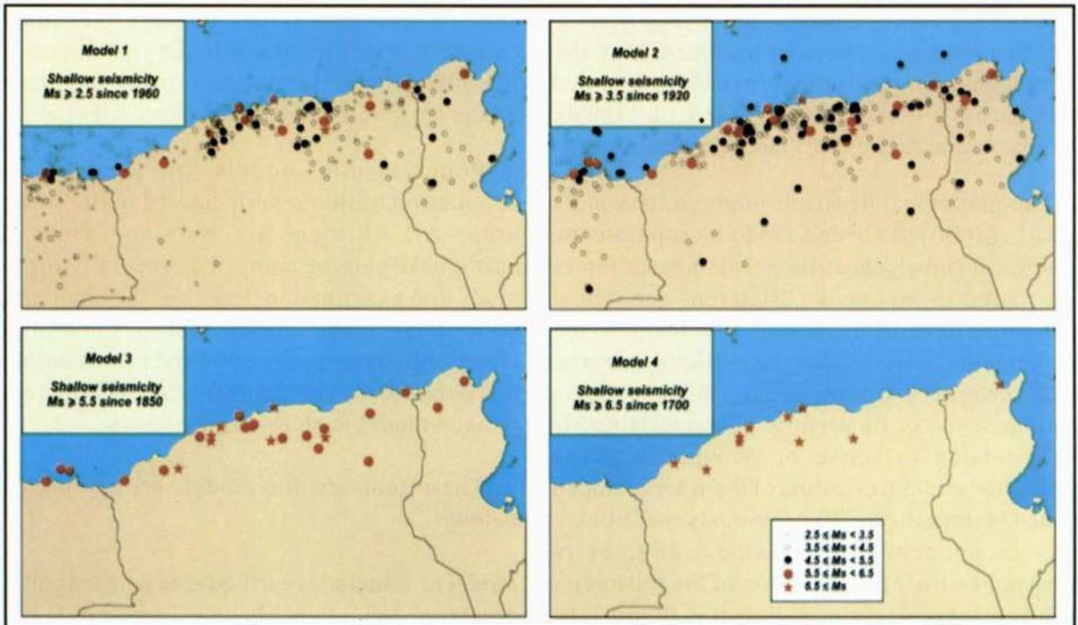
Fig. 4 - Shallow seismicity included in the different models.
