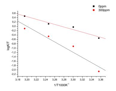
Fig.5. Plot of log (corrosion rate/T) versus  $1/T \times 10^3$ ,  $K^1$  for carbon steel in decanted water Solution in absence and in presence of 300 ppm of inhibitor.
