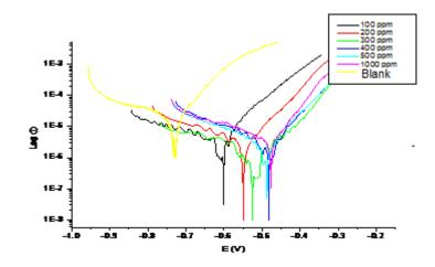
Fig 2: Polarization curves of carbon steel in decanted water in the absence and various concentrations of inhibitor
