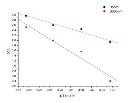
Fig.4. Plot of log (k) versus  $1/Tx10^3$ ,  $K^1$  for carbon steel in decanted water Solution in absence and in presence of 300ppm of inhibitor.
