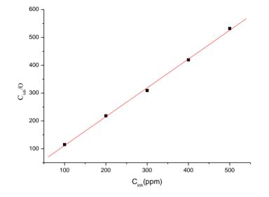
Fig.3. Plot of  $C_{inh}/\Theta$  versus  $C_{inh}$  for carbon steel in decanted water solution in presence of different concentrations of inhibitor
