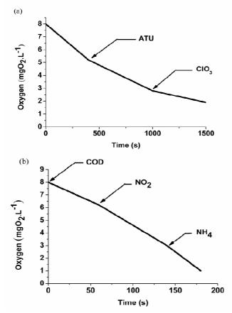
**Figure 1.** Profile of O<sub>2</sub> versus time for determination of biomass activity (a) by inhibitor injection, (b) by specific substrate addition.
