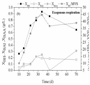
Figure 3. Biomass concentrations ( $X_{BH}$   $X_{BA1}$   $X_{BAA}$ ) in endogenous and exogenous respiration, with ASM1 and ASM3 respiration (SRT= 60d)
