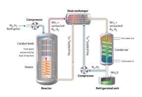
Figure 1. Schematic diagram of an ammonia reactor.
