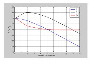
Figure. 3. Profiles of  $N_{N2}$ ,  $T_f$  and  $T_g$  vs Reactor Length
