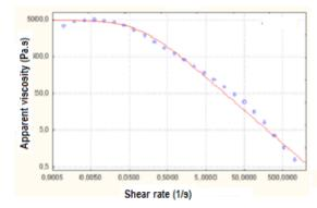
Figure 2.Flow curve of GTW-Hydrogel stored at 4°C for 8 months, T = 20 ° C.
