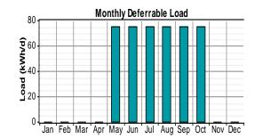
Figure 1. Monthly energy consumption for water pumping
