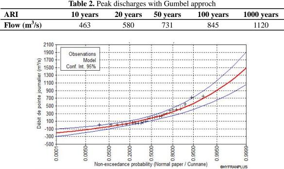
**Fig.8.** Peak discharges adjusted with Gumbel statistical method
