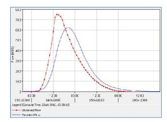
Fig.10. Observed and simulated hydrographs for Ain Sefra watershed in HEC-HMS before calbiration
