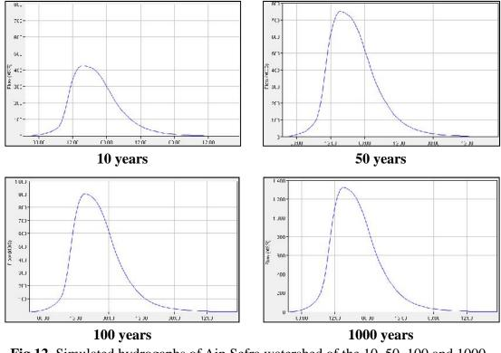
Fig.12. Simulated hydrogaphs of Ain Sefra watershed of the 10, 50, 100 and 1000 return period
