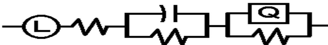
**Fig.4.** Electrical Equivalent circuit model used to fit impedance data
