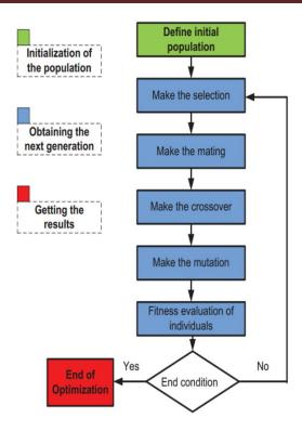
Fig. 3 General mechanism for GA computation
