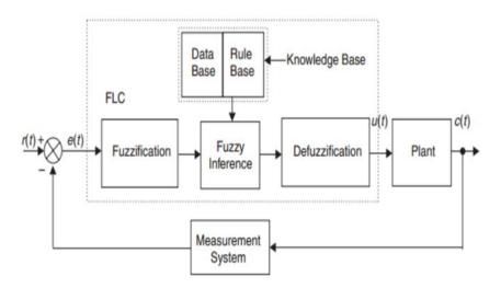
Fig. 1 Block diagram for a fuzzy logic controller
