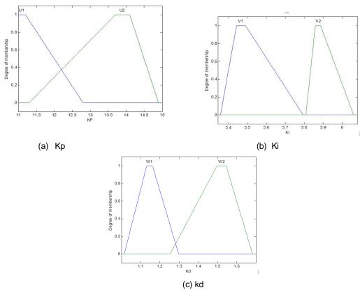
Fig. 9 the membership functions for the fuzzy controller outputs.
