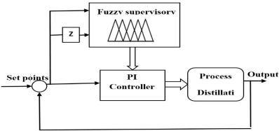
Fig. 2 Block diagram for a PI fuzzy supervisory PI I controller
