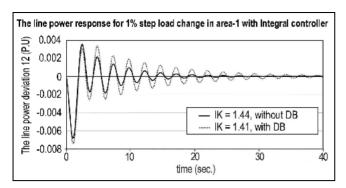
Figure 4: Double area thermal-thermal with and without governor deadband effect.
