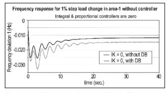
Figure 2: Double area thermal-thermal with and without governor deadband effect.
