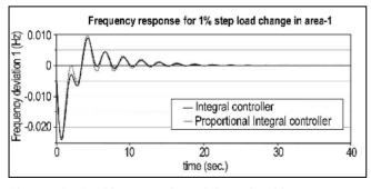
Figure 6: Double area thermal-thermal without governor deadband effect.
