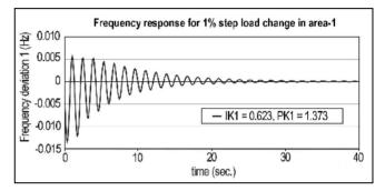
Figure 7: Double area thermal-thermal with governor deadband effect, B = 2.12.
