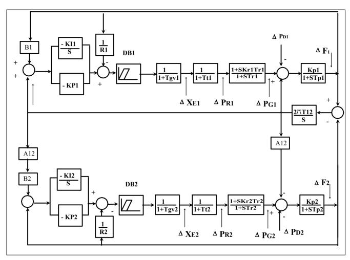
Figure 1: Block diagram for two area (Thermal-Thermal) power system.
