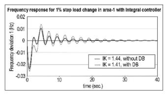
Figure 3: Double area thermal-thermal with and without governor deadband effect.
