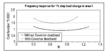
**Figure 5**: Integral controller vers Cost function with beta = 0.424 and A12 = -1.
