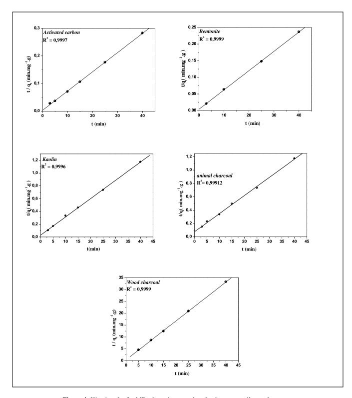
**Figure 4:** Kinetics plot for MB adsorption onto the adsorbents according to the pseudo-second order model.
