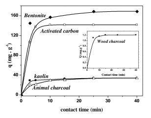
**Figure 1**: Effect of time contact on MB adsorption capacity q (mg/g) on various natural materials.
