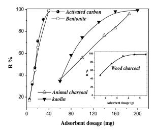
Figure 2: Adsorbent amount effect in MB removal
