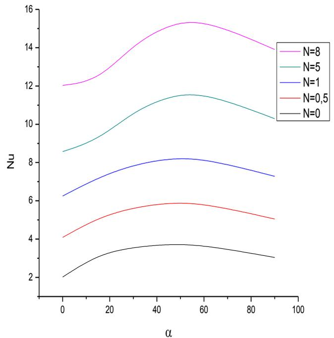
Fig. 5. Global Nusselt number versus inclination angle  $\alpha$  for different values of the Buoyancy ratio  $N$ .
