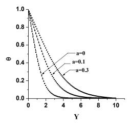
Fig.3 Temperature profiles at X=0.5 for different values of the amplitude wavelength and for m=0
