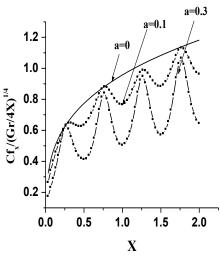
Fig.5 Skin-friction coefficient for different values of the amplitude wavelength and for m=0
