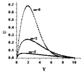
Fig.6 Velocity profiles at X=0.5 for different values of the constant m and for a=0.2
