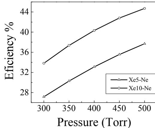
**Figure..8.** The discharge efficiency as a function of the total pressure for two mixtures of gas; Xe5%- Ne and Xe10%-Ne.
