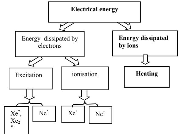
Figure.1. Schematic of the discharge energy deposited in the cell.
