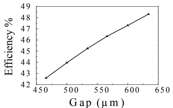
**Figure.5.** Effect of the coplanar electrodes gap on the discharge efficiency.
