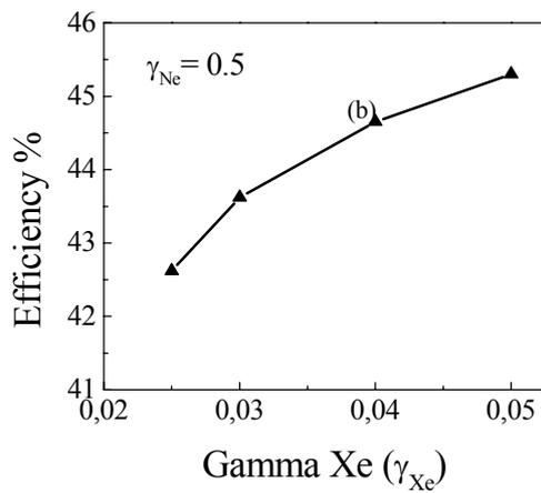
b) the xenon excitation efficiency. The sustain voltage is equal to 290 V. The neon gamma is equal to 0.5.
