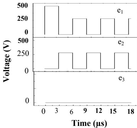
**Figure.3.** Typical driving voltage sequence applied to the cell electrodes.
