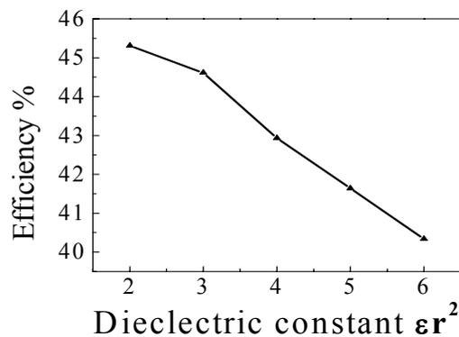
**Figure.7.** The discharge efficiency as a function of the relative permittivity of the dielectric covering the address electrode.
