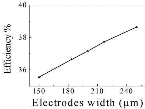
**Figure 6.** Effect of the coplanar electrodes width on the discharge efficiency.
