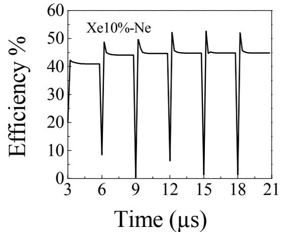
**Figure. 4.** Temporal evolution of the discharge efficiency
