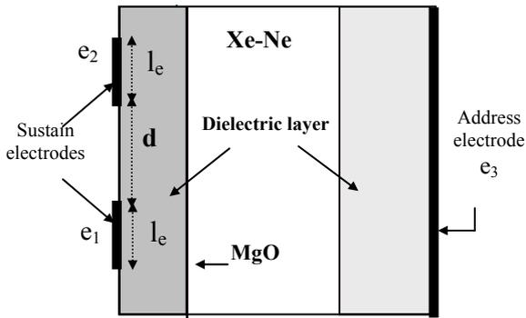
**Figure.2.** A model of the cell geometry is shown schematically.
