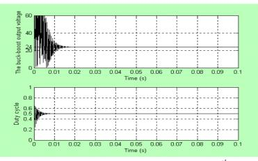
Fig. 6: The generated output voltage and duty cycle in the 3<sup>rd</sup> case
