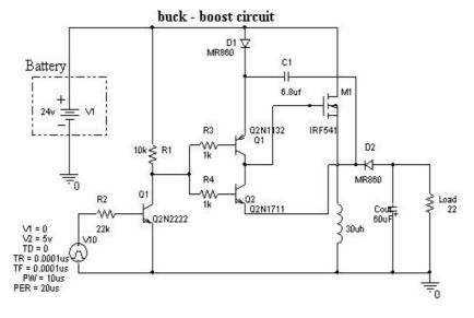
Fig. 2: Load voltage regulator circuit
