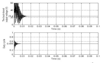
Fig. 5: The generated output voltage and duty cycle in the 2<sup>nd</sup> case
