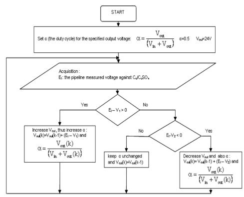
Fig. 7: The cathodic protection control and monitoring algorithm
