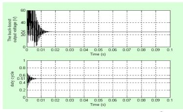
Fig. 4: The buck-boost output voltage and duty cycle in the 1<sup>st</sup> case
