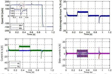
Fig. 5: Performance of vector controlled for five-phase PMSM using PI controllers
