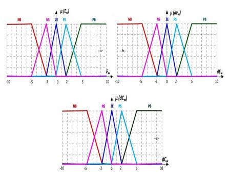
Fig. 2: Membership functions of input/output variables: **a**- input speed error; **b**- input change speed error; **c**- output
