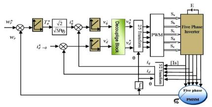
Fig.1: Vector control for the five-phase PMSM
