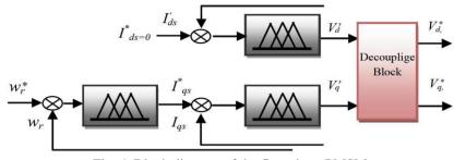
Fig. 4. Block diagram of the five-phase PMSM vector control with the fuzzy controller
