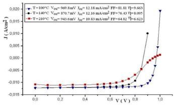
Fig. 3: Illuminated J-V characteristic of a-Si solar cell for different substrate temperature T = 100 °C, 140 °C et 210 °C
