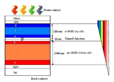
Fig. 6: Schematic structure of micromorph tandem cell in superstrate configuration
