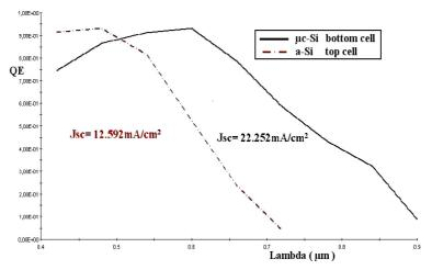
Fig. 7: Spectral response curves of the tandem micromorph cell
