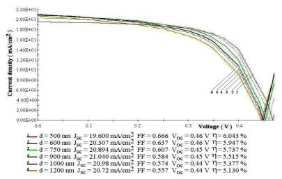
Fig. 5: Influence of intrinsic layer thickness in the performance of µc-Si solar cell
