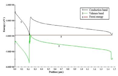
Fig. 8: Band diagram of the tandem cell a-Si/µc-Si in the thermodynamic equilibrium
