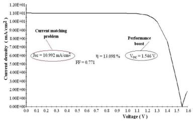
Fig. 9: Illuminated J-V characteristic of micromorph tandem cell
