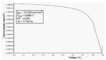
Fig. 2: The illuminated J-V characteristic
