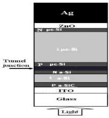
Fig. 1: Schematic view of the typical Micromorph tandem solar cell
