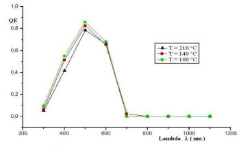
Fig. 4: Quantum efficiency of a-Si solar cell at T = 100 °C, 140 °C and 210 °C
