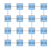
Fig. 12. A regular Mesh with 2D-coordinates
