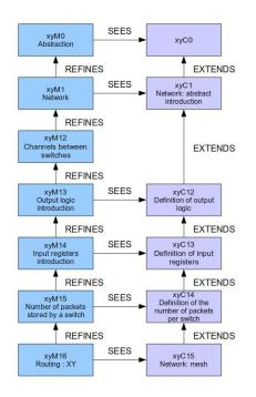
Fig. 5. Step-by-step Modeling of NoC Architecture
