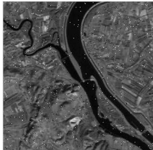
The image comprises a great quantity of data but generally this image is noisy by undesirable pixels which could modify useful information, therefore it is essential to pass by the stage of pretreatment. We apply to the initial image a median filter used to eliminate useless information. Fig.5
