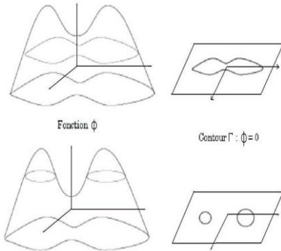
FIG. 2 Representation «level set » of a contour
