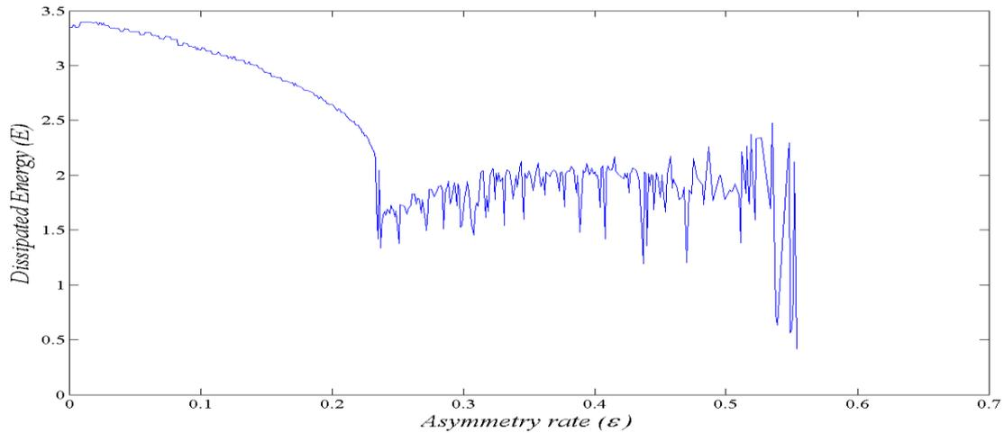
Figure. 11. Energy Assessment of the perfect damped and asymmetric elastoplastic oscillator for:  $\zeta = 0.1$ ;  $f_0 = 0.8$ ;  $\omega = 0.75$
