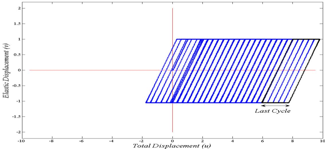
Figure. 9. Behaviour of the perfect damped and asymmetric in compression elastoplastic oscillator ( $F^+ < F^-$ ), “Dynamic ratcheting” for:  $(v_0, u_0) = (0, 0)$ ;  $\zeta = 0.1$ ;  $\omega = 0.75$ ,  $f_0 = 0.8$ ,  $\varepsilon = 0.05$
