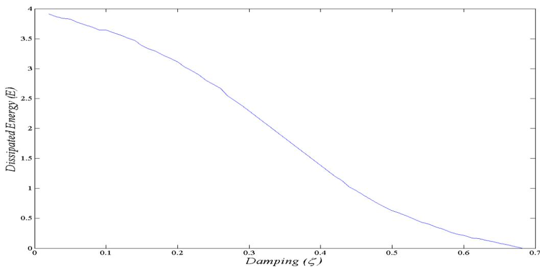
Figure.6: Energy Assessment for the perfect damped and symmetric elastoplastic oscillator for:  $(\mathbf{v}_0, \mathbf{u}_0) = (\mathbf{0}, \mathbf{0}); \omega = 0.5; f_0 = 1$
