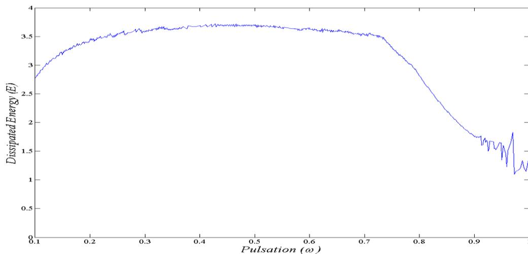
Figure.10: Energy Assessment of the perfect damped and a symmetric elastoplastic oscillator for :  $\zeta = 0.1$ ;  $f_0 = 0.8$ ;  $\varepsilon = 0.05$
