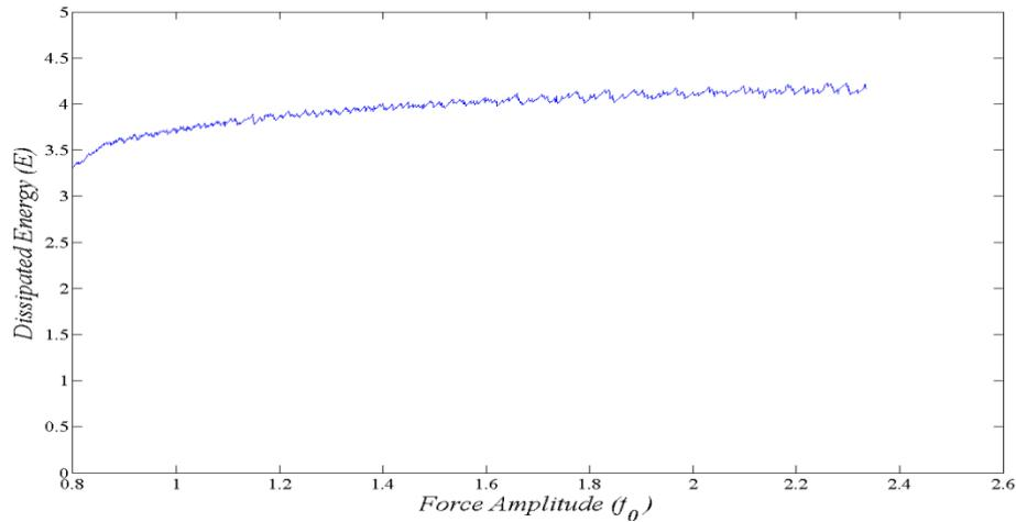
Figure. 13. Energy Assessment of the perfect damped and asymmetric elastoplastic oscillator for : $\varepsilon = 0.05$ ;  $\zeta = 0.1$ ;  $\omega = 0.75$
