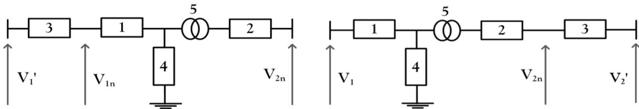
a) When the regulator is placed at the primary      b) When the regulator is placed at the secondary
