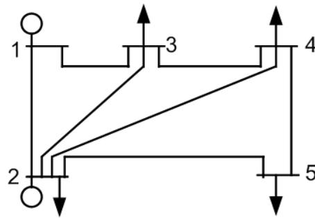
**Figure 4:** Five nodes test-network
