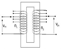
**Fig.1:** Diagram showing a transformer with load regulation
