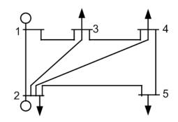
Figure 4: Five nodes test-network
