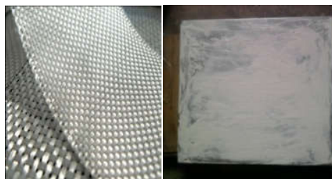
Fig. 2 – Preparation of the composite: weighing of the hardener, coating of the gel-coat mold, then deposition of the fiberglass.
