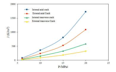
Fig. 6b– Evolution of the integral J as a function of the load P ( $\phi$ =90, a/t =0.33 and a/c=0.75).
