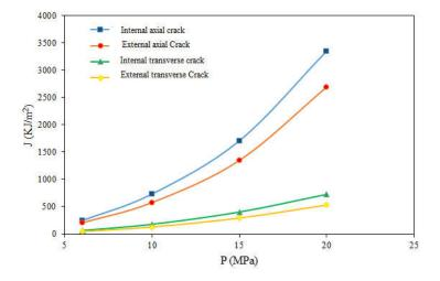
Fig. 6a– Evolution of the integral J as a function of the load P ( $\phi=0$ , a/t =0.33 and a/c=0.75).
