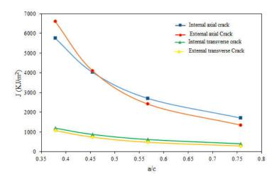
Fig. 11– Evolution of the integral J as a function of the a / c ratio ( $\phi=0$ ; a/t=0.33 P=15 MPa).
