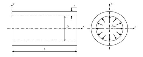
Fig. 2 – Schematic representation of a pipe under internal pressure P.
