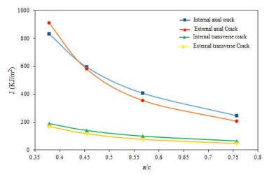
Fig. 7– Evolution of the integral J as a function of the a / c ratio ( $\phi=0$ ; a/t =0.33 P= 6 MPa).
