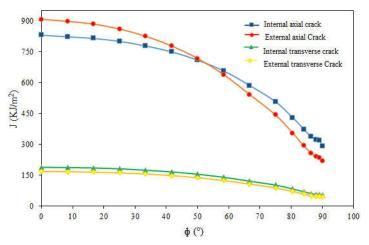
Fig. 5d– Evolution of the integral J as a function of the orientation angle (a / t = 0.66).
