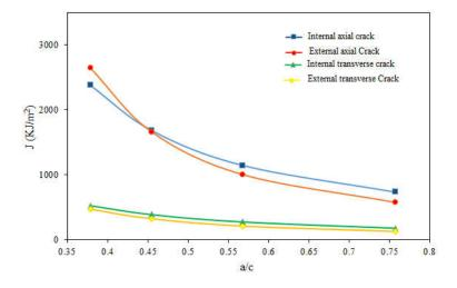
Fig. 9– Evolution of the integral J as a function of the a / c ratio ( $\phi=0$ ; a/t=0.33 P=10 MPa).
