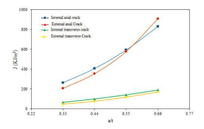
Fig. 15– Evolution of the integral J as a function of the a/t ratio ( $\phi$ =0).
