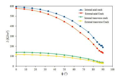
Fig. 5c– Evolution of the integral J as a function of the orientation angle (a / t = 0.55).
