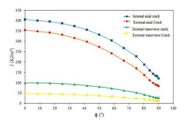
Fig. 5b– Evolution of the integral J as a function of the orientation angle (a / t = 0.44).
