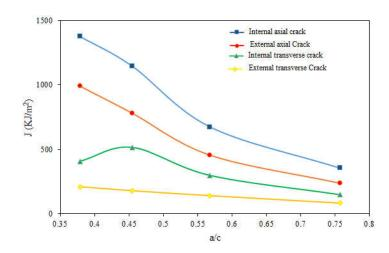
Fig. 10– Evolution of the integral J as a function of the a / c ratio ( $\phi=90$ ; a/t=0.33 P=10 MPa).
