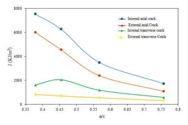
Fig. 14– Evolution of the integral J as a function of the a / c ratio ( $\phi$ =90; a/t =0.33 P= 20 MPa).
