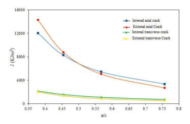
Fig. 13– Evolution of the integral J as a function of the a / c ratio ( $\phi=0$ ; a/t = 0.33 P = 20 MPa).
