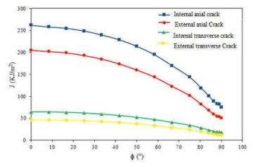
Fig. 5a– Evolution of the integral J as a function of the orientation angle (a/t = 0.33).
