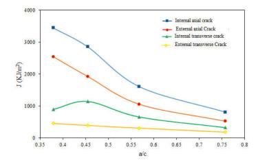
Fig. 12– Evolution of the integral J as a function of the a / c ratio ( $\phi=90$ ; a/t=0.33 P=15 MPa).
