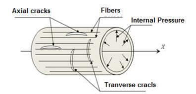
Fig. 1 – Representation of pipe with axial and transverse cracks.
