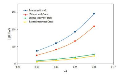
Fig. 16– Evolution of the integral J as a function of the a/t ratio ( $\phi$ =90).
