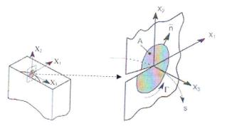
Fig. 4- Representation of the J integral in 3 dimensions
