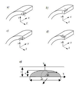
Fig. 3 – Cracks studied. a) Internal axial crack (IAC), b) External axial crack (EAC), c) Internal transverse crack (ITC), d) External transverse crack (ETC) e) Shape of the crack.
