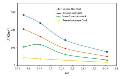
Fig. 8– Evolution of the integral J as a function of the a / c ratio ( $\phi=90$ ; a/t=0.33 P=6 MPa).
