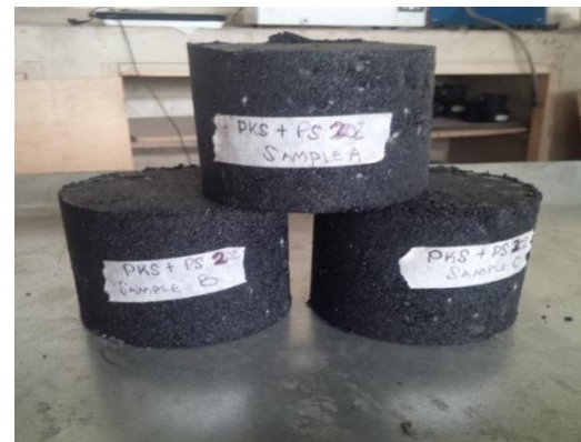
Fig 6. Marshall stability test specimen (PWS)
