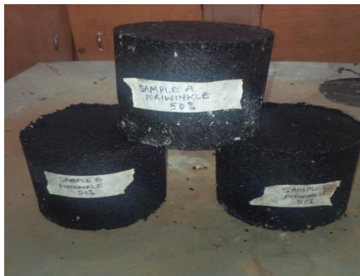
Fig 5. Marshall stability test specimen (PKS)
