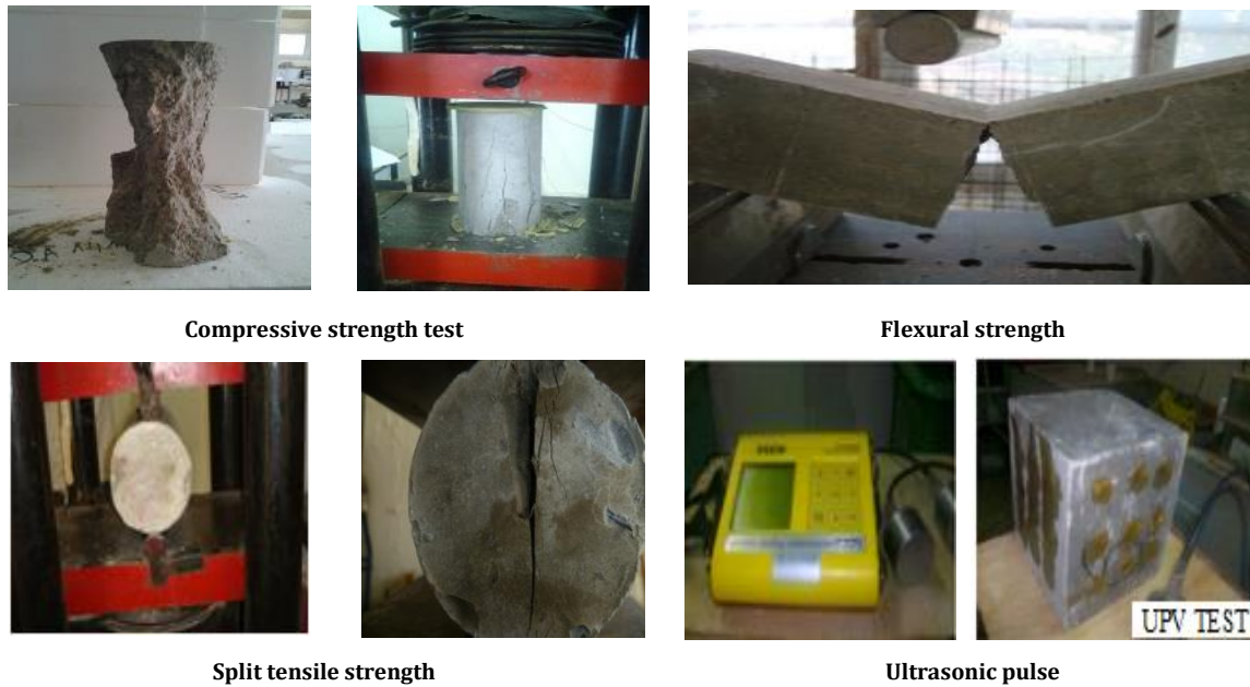
Fig 7. Hardened tests on SCC.
