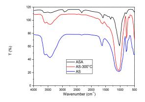
*Figure 2. FTIR spectra of AS, AS-300°C and ASA.*
