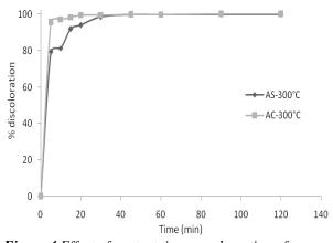
*Figure 4.*Effect of contact time on adsorption of methylene blue by AC-300°C and AS-300°C.
