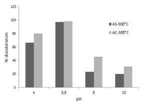
*Figure 5.Effect of pH on adsorption of methylene blue by AC-300°C and AS-300°C.*
