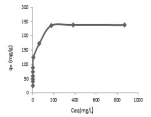
*Figure 7.* Adsorption isotherm of methylene blue onto AS-300°C
