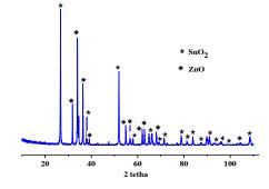
*Figure 2.* The XRD pattern of ZnO-SnO<sub>2</sub> prepared by nitrate route.
