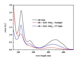
**Figure 4.** The influence of the light intensity on the ARS photodegradation (ARS= 20 mg/L, pH= 9, T = 25 °C and catalyst dose = 0.5g/L).
