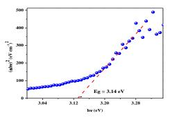
**Figure 3.** The direct optical transition of the ZnO-SnO<sub>2</sub>.
