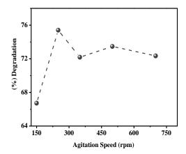
**Figure 6.** Effect of the stirring speed on the photodegradation ( $C_o$ : 20 mg/L; catalyst dose: 0.5 g/L; pH~9)
