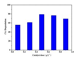
**Figure 5.** Histogram showing the influence of  $ZnO-SnO_2$  dose on the photoactivity: ( $C_o$ : 20 mg/L, temperature: 298 K, reaction time: 180 min, pH ~ 9 and stirring speed: 250 rpm).
