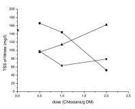
**Figure 5.** Variation of filtrate suspension matter with chitosan dose for each flocculant RSDMDA7dT30 ( $\bigstar$ ), RSDA7dT30 ( $\blacktriangle$ ) and ChitosCom( $\blacksquare$ )
