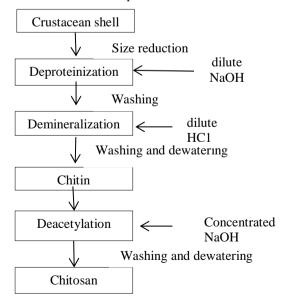
Figure 1. Conventional diagram of chitin and chitosan processing [4].
