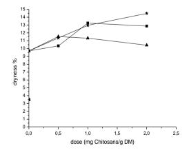
*Figure 2.* Variation of cake dryness with chitosan dose for each flocculant RSDMDA7dT30 (¥), RSDA7dT30 (▲) and ChitosCom (■).
