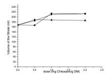
**Figure 3.** Variation of filtrate volume with chitosan dose for each flocculant RSDMDA7dT30 ( $\bigstar$ ), RSDA7dT30 ( $\blacktriangle$ ) and ChitosCom ( $\blacksquare$ ).
