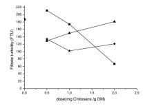
**Figure 4.** Variation of filtrate turbidity with chitosan dose for each flocculant RSDMDA7dT30 ( $\bigstar$ ), RSDA7dT30 ( $\bigstar$ ) and ChitosCom ( $\square$ )
