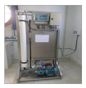
Fig1. Reverse Osmosis pilot installed in the DDEMS laboratory
