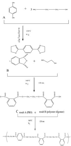
Schema 1: A) Synthesis of bisoxazoline with polycondensation method, B) polyester oligomer, C) coupling reaction between polyester oligomer  $\omega$   $\omega$ 'diacides and PBO.
