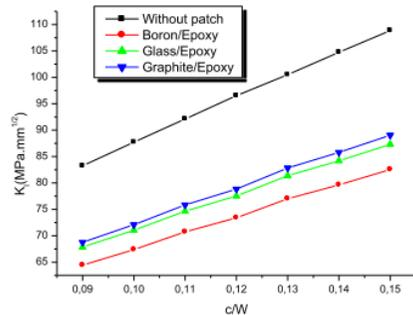
**Fig.12.** Stress intensity factor (SIF) vs. ratio  $c/W$  for external position of crack-front, for different composites.
