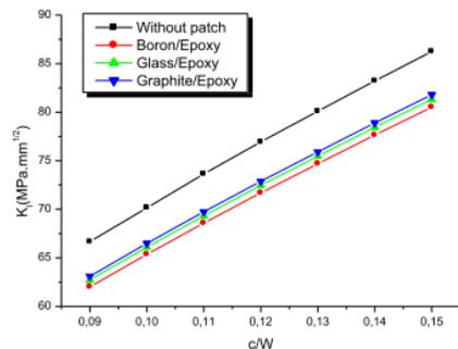
**Fig. 13.** Stress intensity factor (SIF) vs. ratio  $c/W$  for internal position of crack-front, for different composites
