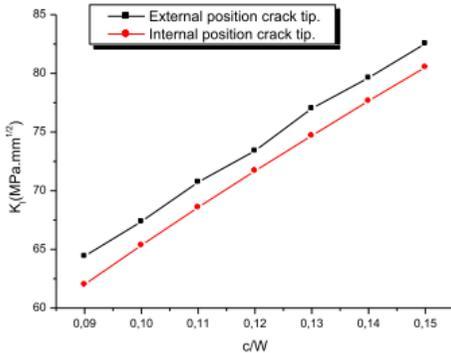
**Fig.7.** Stress intensity factor (SIF) vs. ratio  $c/W$  for internal and external position of crack-front
