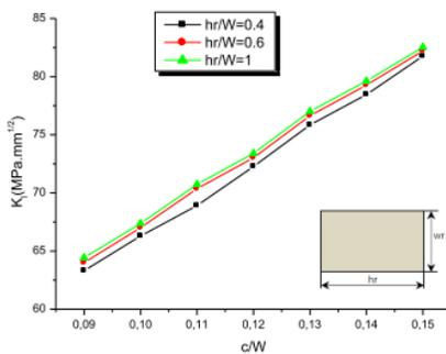
**Fig. 11.** Effect of the patch area on the variation of the SIF for external position of crack-front
