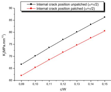
**Fig. 6.** Variation of the SIF  $K_I$  according to the ratio  $c/W$  for internal position of crack-front patched and unpatched ( $\alpha=\pi/2$ ).
