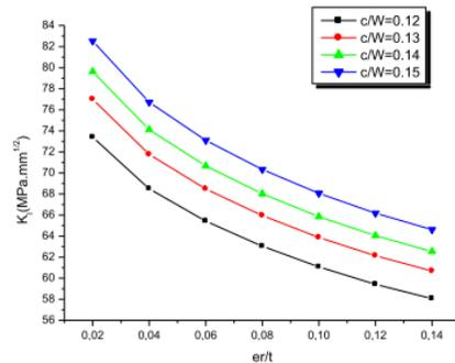
**Fig. 9.** Effect of the patch thickness on the variation of the SIF for external position of crack-front
