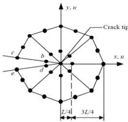
**Fig. 1** Quarter-point singular elements around the crack tip
