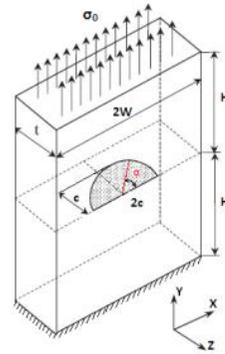
**Fig. 2** Semi-circular surface crack in a finite-thickness with Boundary conditions and loading applied
