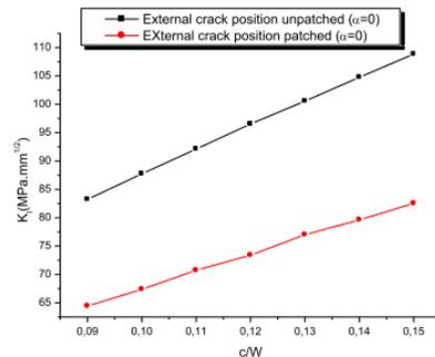
**Fig. 5.** Variation of the SIF  $K_I$  according to the ratio  $c/W$  for external position of crack-front patched and unpatched ( $\alpha=0$ ).
