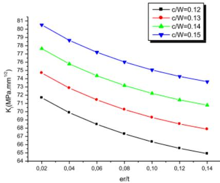
**Fig. 10.** Effect of the patch thickness on the variation of the SIF for internal position of crack-front
