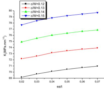
**Fig. 8.** Stress intensity factor (SIF) vs. ratio ( $ea/t$ ) for internal position of crack-front
