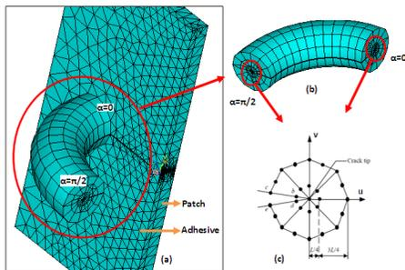
**Fig. 4.** Typical mesh model: (a) between the external position crack tip, adhesive layer and composite patch layer; (b) around the crack-front; (c) special elements used for displacement extrapolation method.
