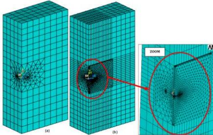
**Fig. 3.** FE model of the semi-circular surface cracks in finite-thickness plates: a) without patch, b) with patch
