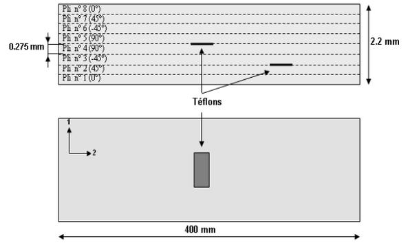
Fig 2. Typical location and size of delaminations
