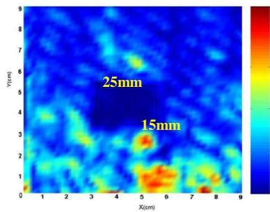
Fig 7.C-scan image of delamination
