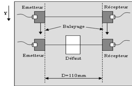
Fig 5. Schematic representation of line-scanning method
