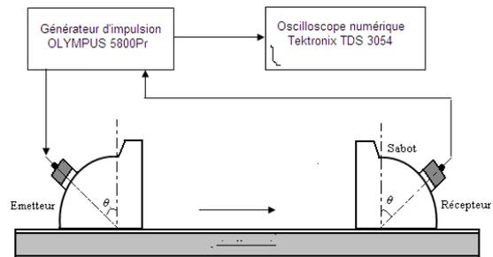
Fig 3:  $S_0$  Lamb wave mode generation and detection.
