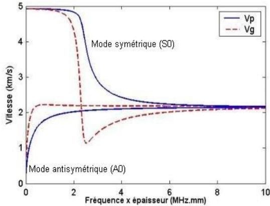
Fig 1. Dispersion curves for an 8 layer laminate composite
