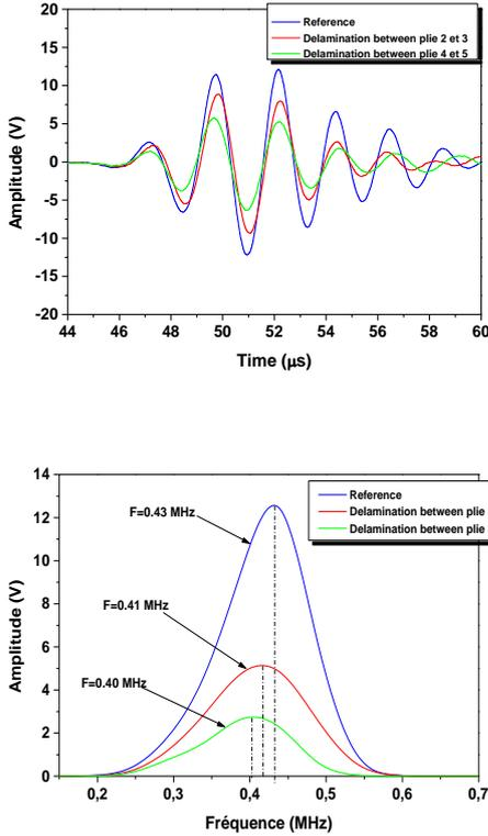
Fig 4: Waveform detected of two different delaminations
