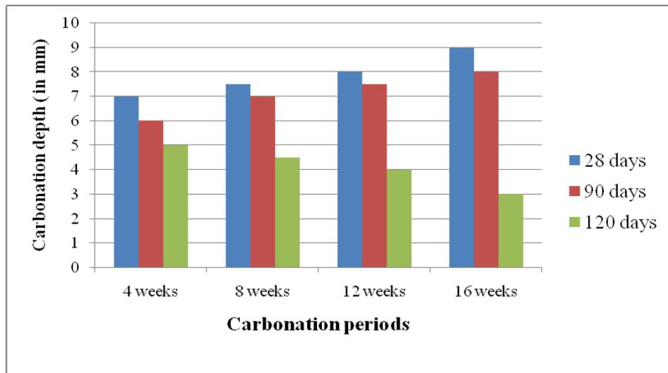
Fig.7- Carbonation depths for HPC mix with 85% cement + 15% MK + 0% CS
