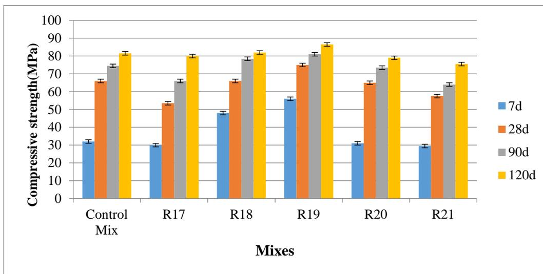
Fig. 2- Compressive strength values of different mixes with varying copper slag%
