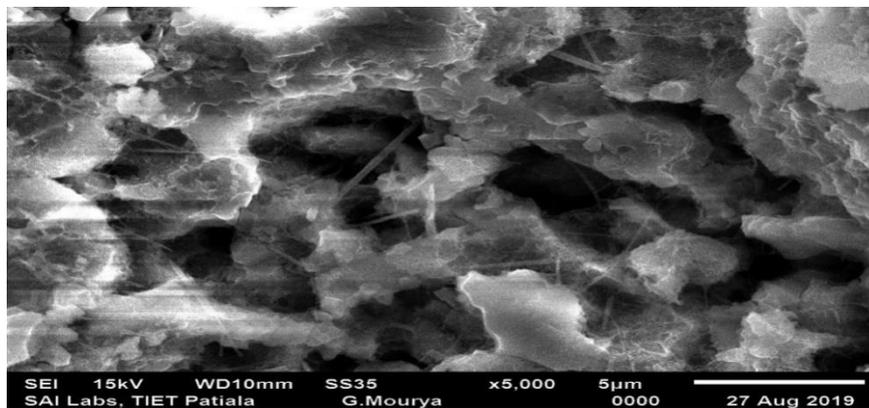
*Fig. 12(f). SEM analysis after 120 days of HPC mixes: (f) R21*
