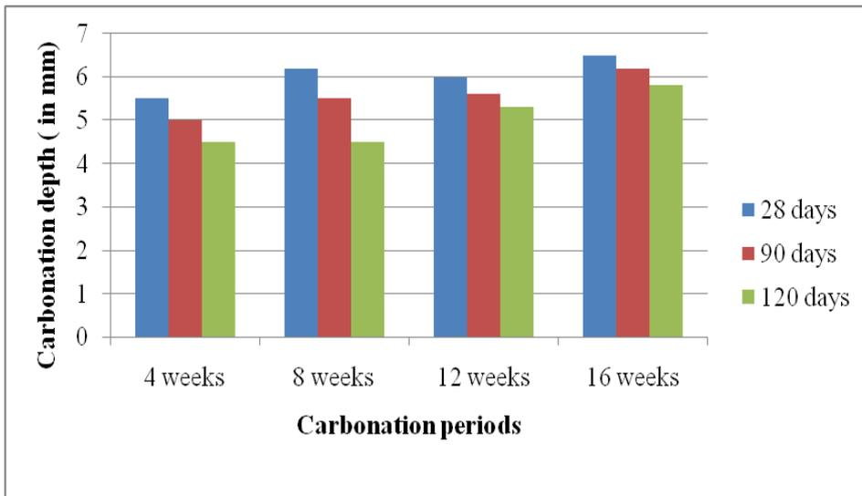
Fig. 10- Carbonation depths for HPC mix with 85% cement + 15% MK + 75% CS
