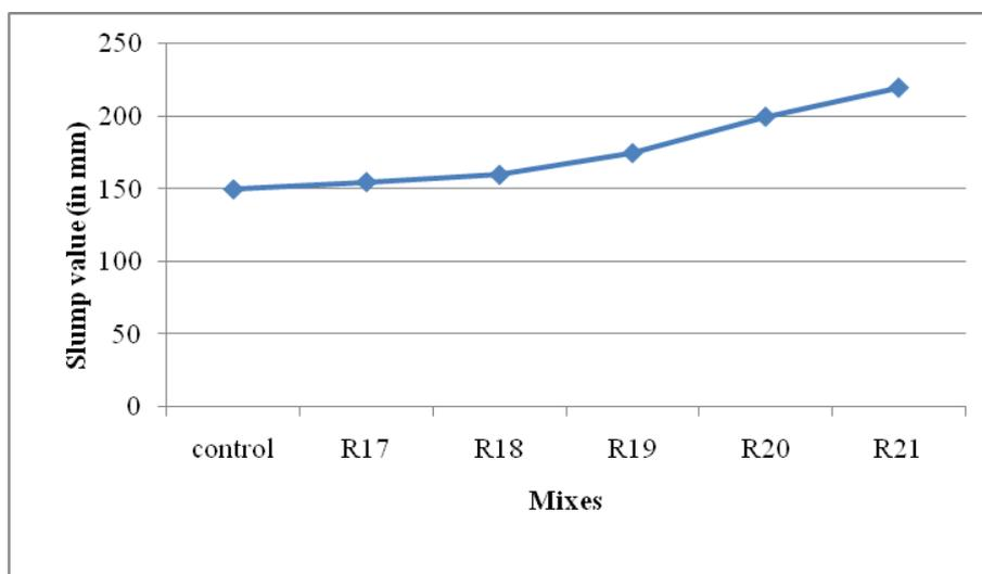
**Fig. 1- Comparison of slump values of different mixes with varying copper slag %**
