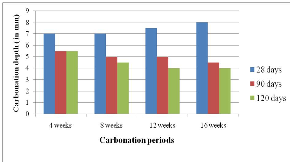
Fig.8- Carbonation depths for HPC mix with 85% cement + 15% MK + 25% CS
