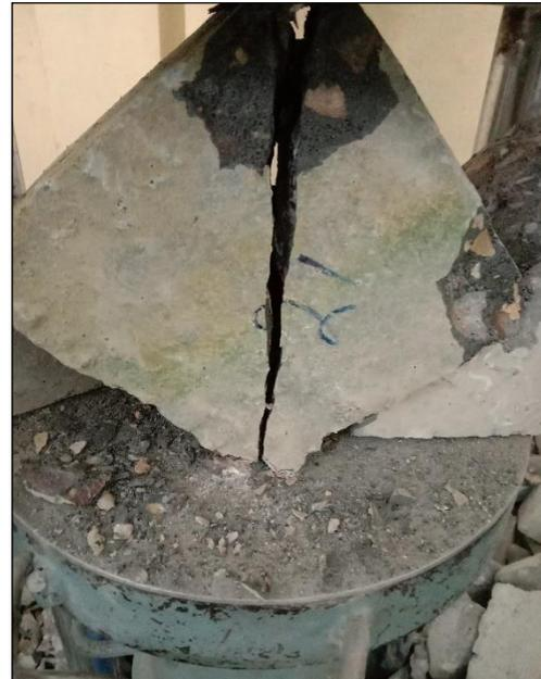
Fig. 4-(b) Splitting tensile strength test
