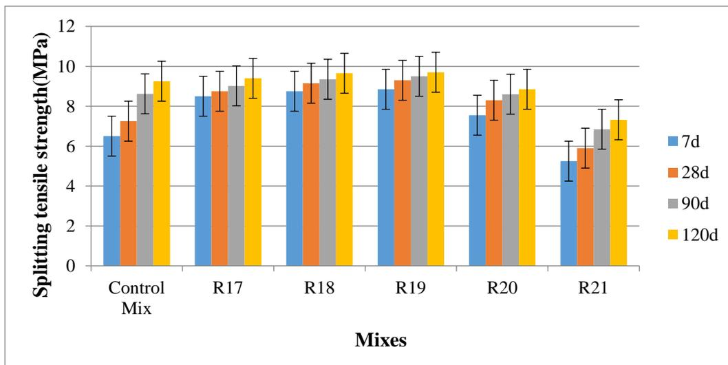
Fig. 3- Splitting tensile strength values of different mixes with varying copper slag %
