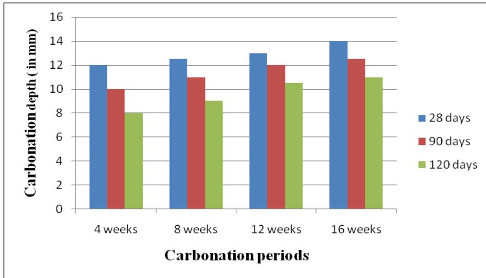
Fig.6- Carbonation depths for HPC Control mix
