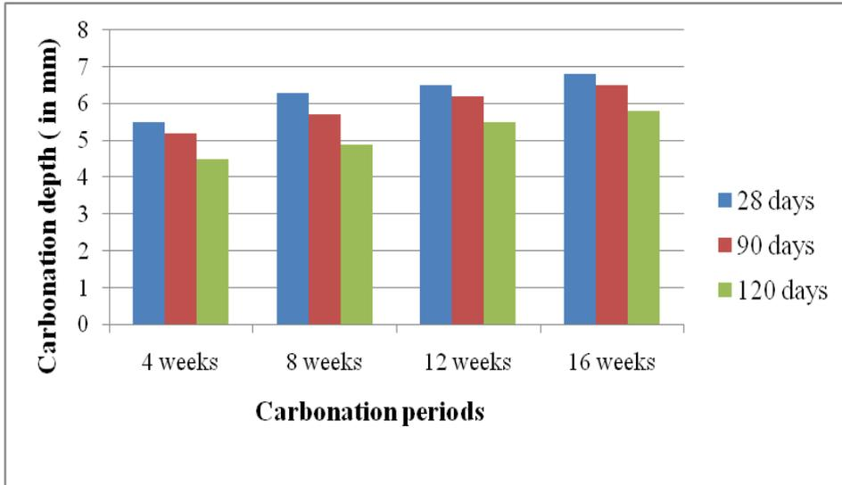
Fig. 9- Carbonation depths for HPC mix with 85% cement + 15% MK + 50% CS
