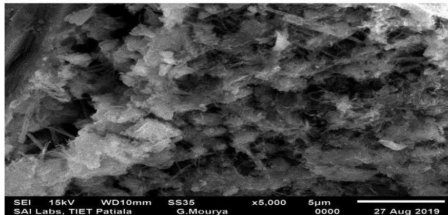
*Fig. 12(a). SEM analysis after 120 days of HPC mixes: (a) R1*
