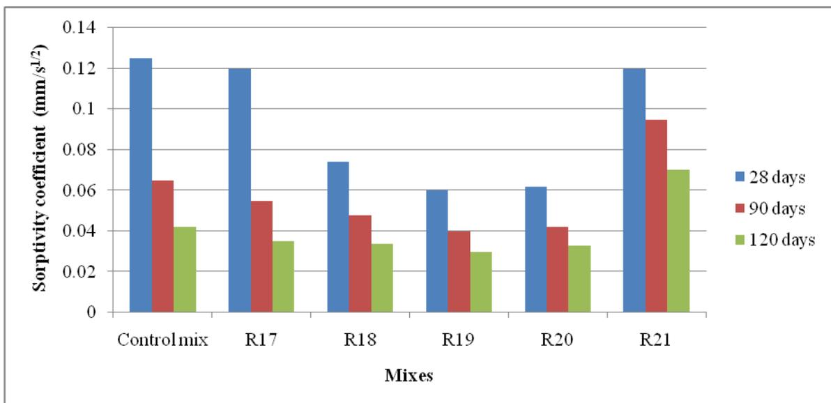
Fig.5- Sorptivity coefficients of various mixes
