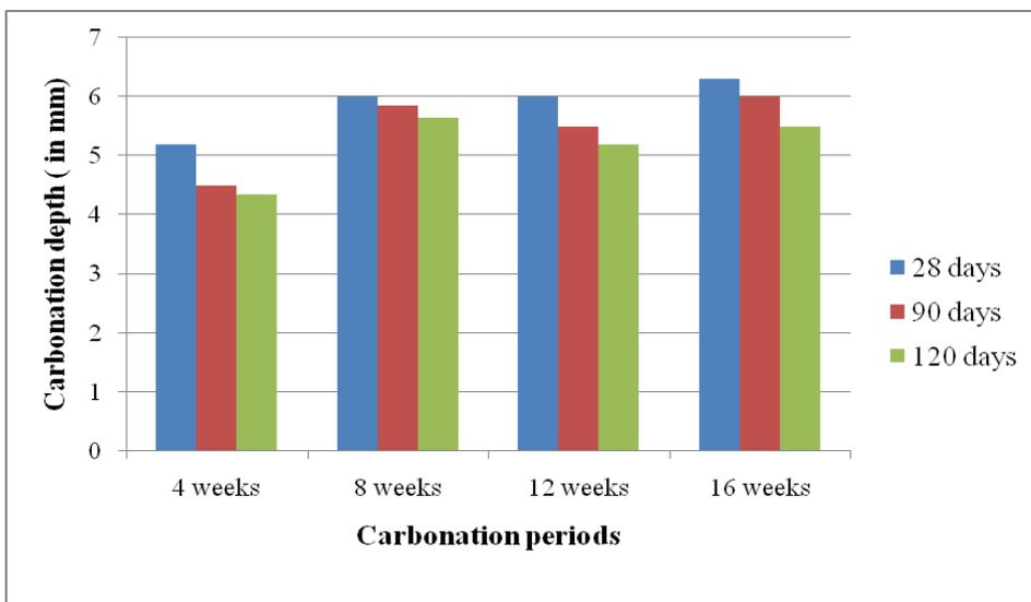
Fig. 11- Carbonation depths for HPC mix with 85% cement + 15% MK + 100% CS
